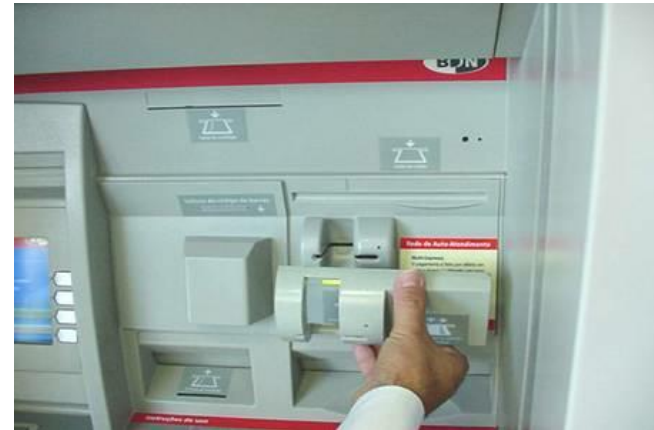
Skimming equipment installed
